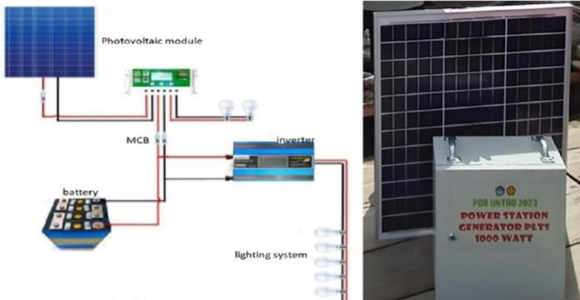
**Gambar 2.3.** PV Portable Generator (Rahman, Y. A., dkk. (2023)
